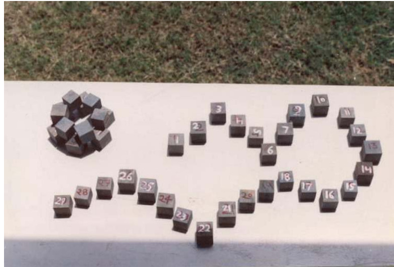
Fig. 2: Rock cubes preparation for measurement of uniaxial compressive strength (JCS)
